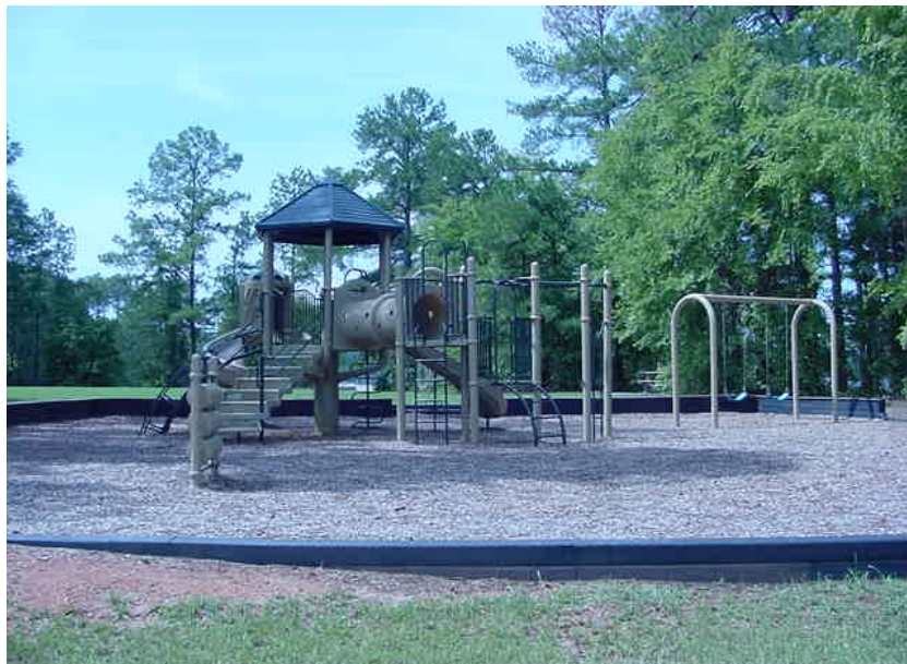
Photo Q-4. Playground features. West Dam Day Use Area, J. Strom Thurmond, GA. Playground has edge material that raises finished grade a minimum of 6", wood fiber play surface, and approximately 50% of the area is shaded ( Table 5.15 )
