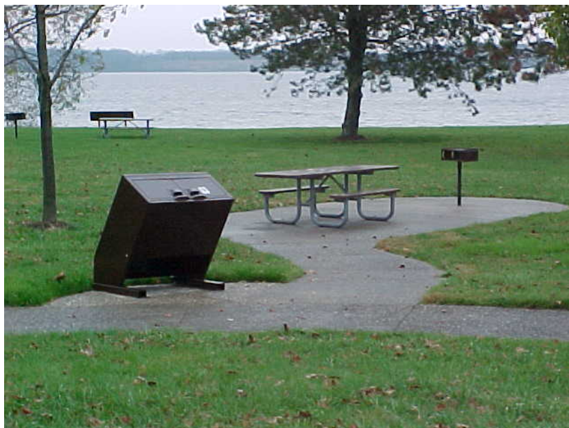
Photo I-7. C.J. Brown Dam and Reservoir, OH. Trash receptacle provided close to high use facilities, Example 2. Double unit doors are animal proof design. Receptacle is UA based on height, and the fact that the doors open to the side instead of being lifted up ( Table 2.8 )
